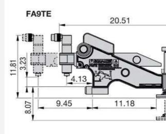
The FA9TE Hydraulic Linear & Rotational Flange Alignment Tool is a simple solution to large-diameter high-pressure flange joint misalignment.
