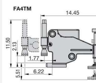
The FA4TM Mechanical Linear & Rotational Alignment Tool is a simple solution to medium-diameter, medium-pressure flange joint misalignment.
